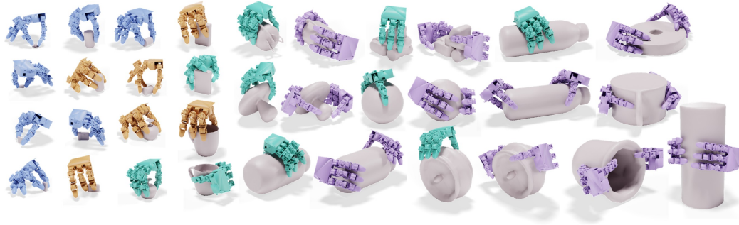
Figure 17: Synthesized LEAP Hand grasps across object scales and contact modes.
