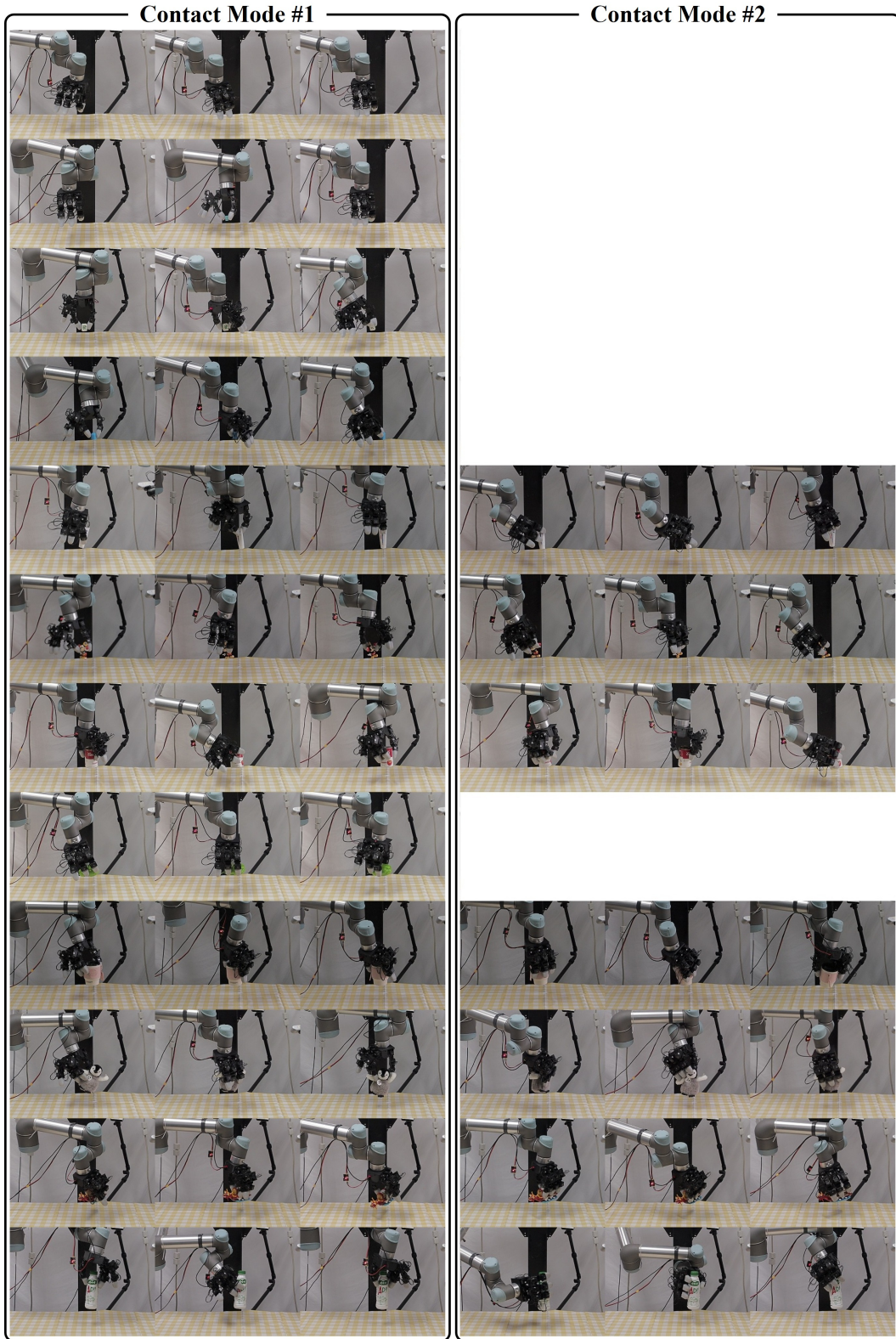
Figure 22: Snapshots of real-world grasp on objects #1–#12. Objects are approximately ordered by increasing scale from top to bottom. Some objects allow only one feasible contact mode, whereas others allow two. For each feasible contact mode, we execute three distinct grasps.
