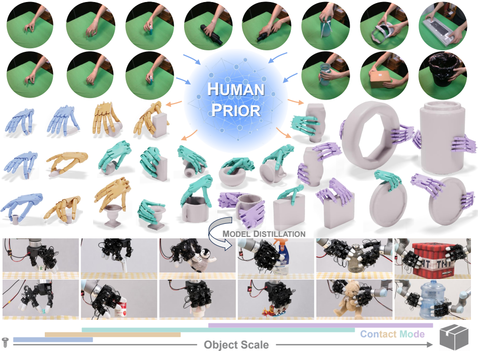
Figure 1: Human priors guide scalable dexterous grasp synthesis across modes and scales. HUGS learns an object-conditioned human prior from a compact self-collected dataset to predict preferred contact modes and wrist initializations. Guided by this prior, force-closure-aware optimization synthesizes diverse and stable grasps ranging from two-finger pinches to bimanual grasps.
